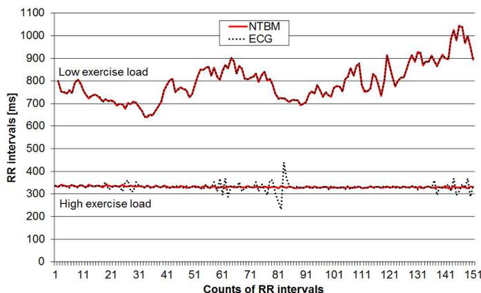
**Figure 3.** Example of 150 RR intervals during low and high exercise conditions, red line describes the RR intervals measured with the NTMB and the black points the RR intervals measured with the ECG
